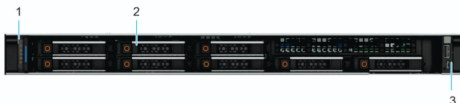
Figure 2. Front view of 8 x 2.5-inch drive system
