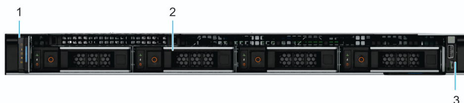
Figure 1. Front view of 4 x 3.5-inch drive system
